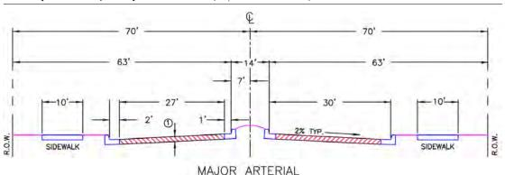
Figure 8: Major Arterial Typical Cross Section
