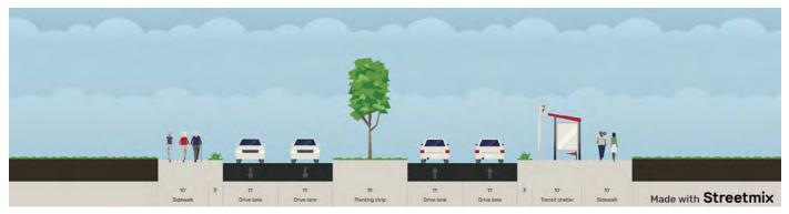
Figure 47: Existing and Proposed Cross Sections for Washington Street
