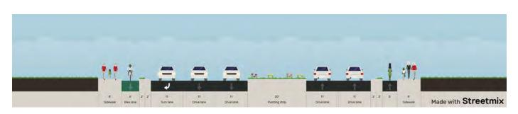
Figure 42: Potential Cross Section on Pecos Street North of 64th Avenue
