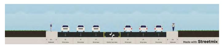
Figure 44: Existing Cross Section of Washington Street Between 73rd Avenue and 78th Avenue
