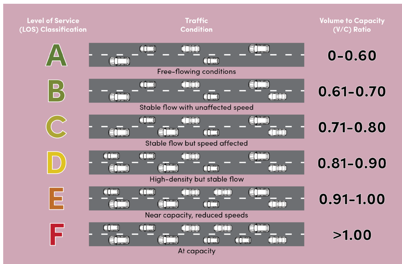
Figure 2.5: Level of Service and Volume to Capacity Ratio Concept (source: Fehr & Peers)
