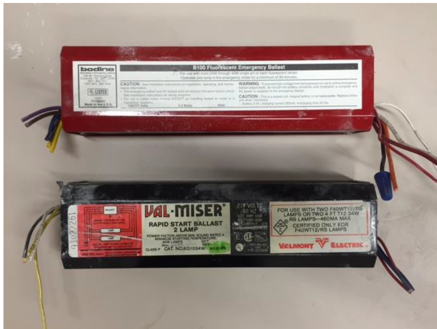
Typical light ballasts with potentially containing PCB or DEHP.
