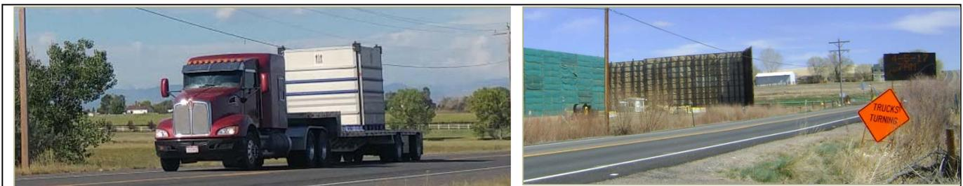
Figure 6. Typical sand truck and traffic control signage for well pad. Trucks slowing down to turn is one of the primary concerns, and the “Trucks Turning” sign alerts drivers to the change in traffic pattern.
