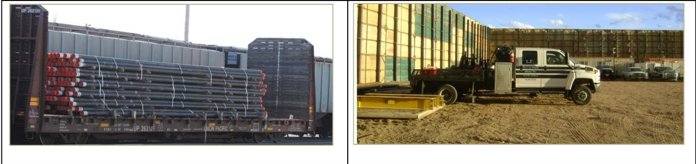
Figure 8. Casing is delivered by rail and transloaded to trucks. Specialized trucks like the one shown at right are used during installation.
