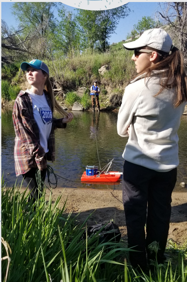
2019 at Clear Creek & Huron St. - ADCP (Acoustic Doppler Current Profiling)
