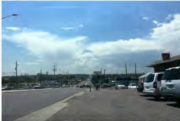
A recent picture of Federal Boulevard looking south. Extensive curbs, head-in parking, limited landscaping, lack of street trees do not provide a pedestrian friendly environment.
