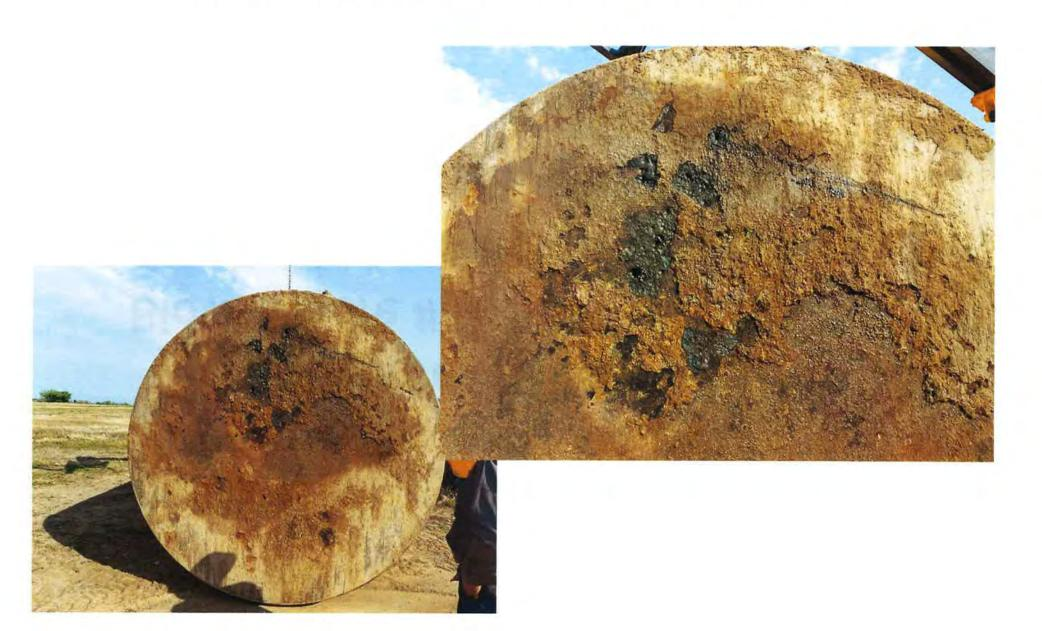
Oil under tank had minimal saturation into the ground. Clay content in the soil appears to have kept the oil in the depression under the tank.
