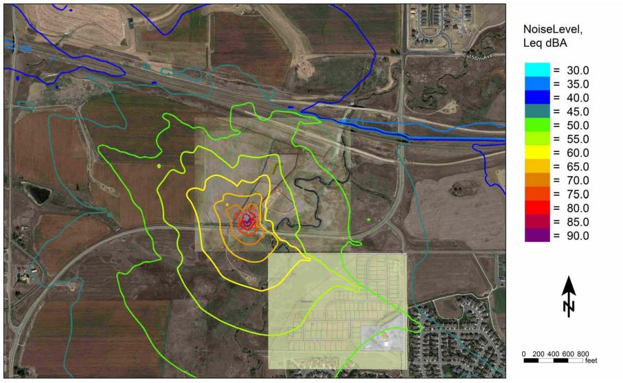
Figure 4-7 Unmitigated Drilling Location 2 Noise Contour Map (dBA)
