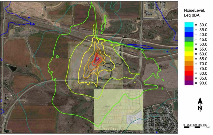
Figure 4-17 Mitigated Drilling Location 1Noise Contour Map (dBA)
