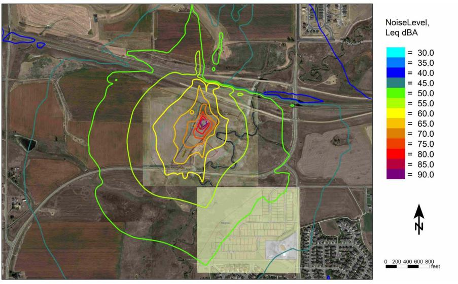
Figure 4-5 Unmitigated Drilling Location 1 Noise Contour Map (dBA)
