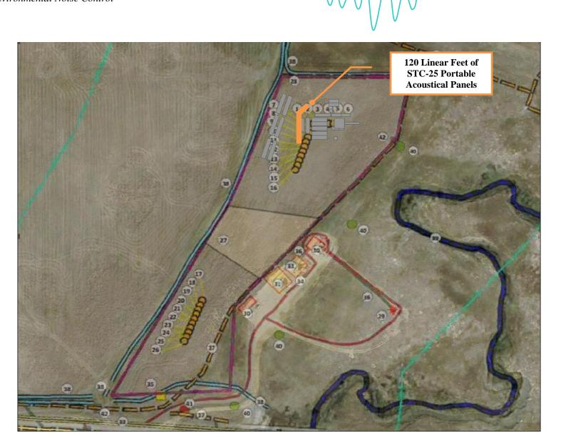
Figure 4-13 Modeled Mitigated Drilling Scenario Layout Location 1
