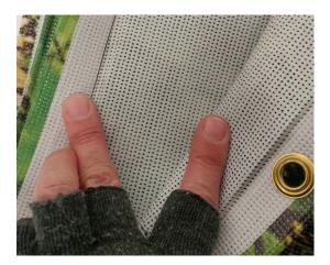
FIGURE 5. DERRICK WRAP MATERIAL.
