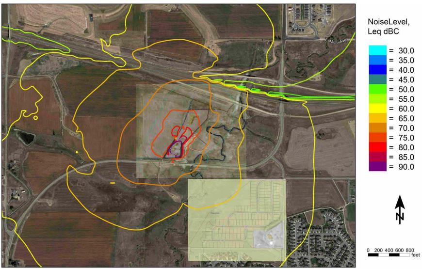
Figure 4-24 Mitigated Fracing Location 2 Noise Contour Map (dBC)
