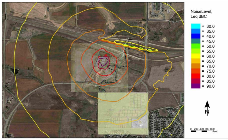
Figure 4-10 Unmitigated Fracing Location 1 Noise Contour Map (dBC)
