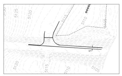
Figure 13.Conceptual sketch of proposed turn lane. Existing one foot contours are shown with labels every five feet. Proposed grading is not shown. The existing access is not shown: it is southeast of the pad. The turn lane and associated grading will be above the 5103' floodplain.
