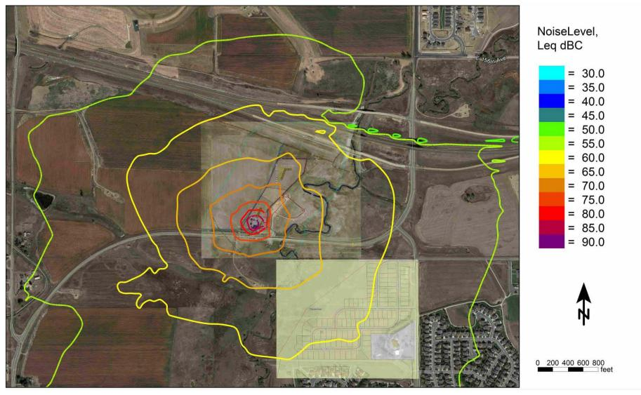
Figure 4-20 Mitigated Drilling Location 2 Noise Contour Map (dBC)
