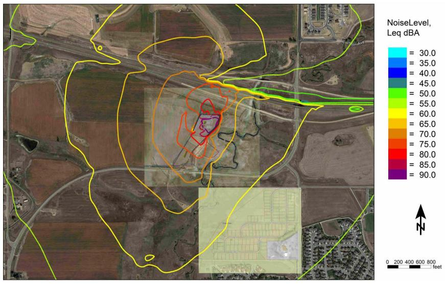
Figure 4-21 Mitigated Fracing Location 1 Noise Contour Map (dBA)
