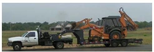
Figure 12. Example of a pickup delivering equipment. Note that the pickup also has a welding set-up mounted on the back.
