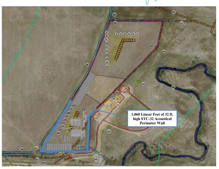
Figure 4-16 Modeled Mitigated Fracing Scenario Layout Location 2
