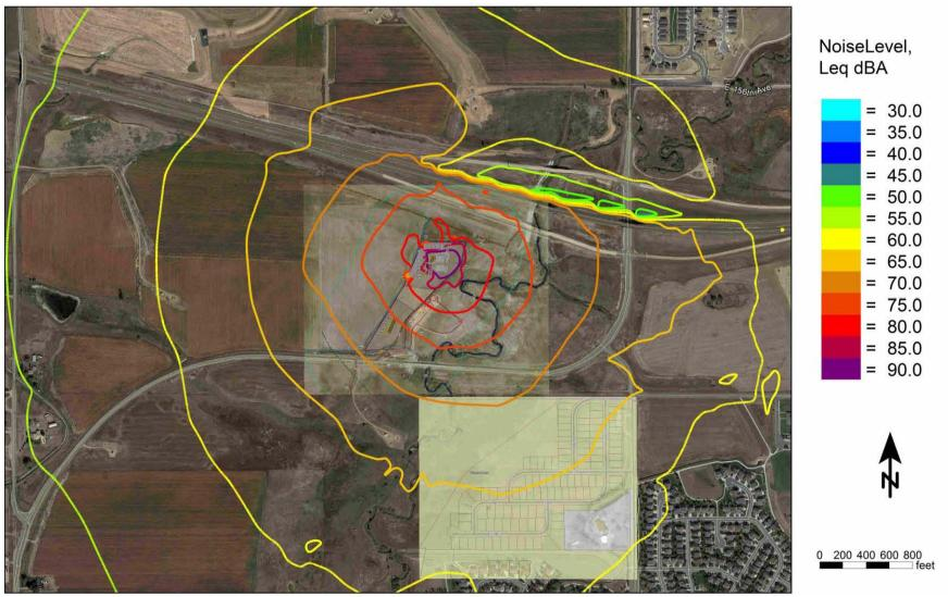
Figure 4-9 Unmitigated Fracing Location 1 Noise Contour Map (dBA)
