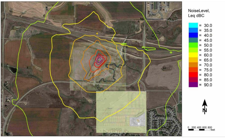
Figure 4-6 Unmitigated Drilling Location 1 Noise Contour Map (dBC)
