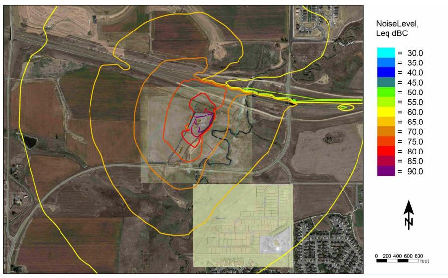
Figure 4-22 Mitigated Fracing Location 1 Noise Contour Map (dBC)
