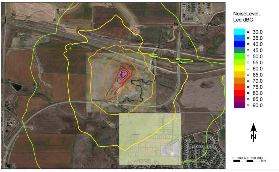
Figure 4-18 Mitigated Drilling Location 1 Noise Contour Map (dBC)
