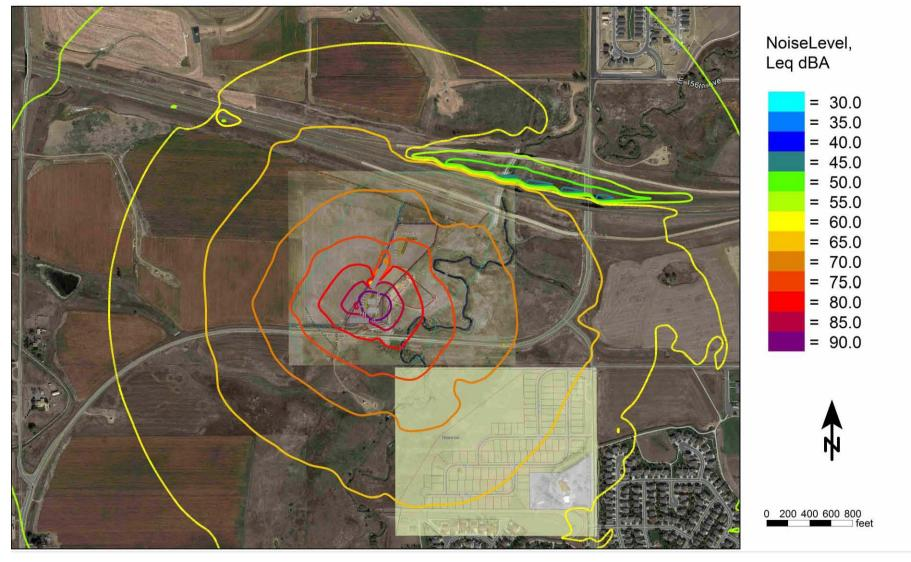
Figure 4-11 Unmitigated Fracing Location 2 Noise Contour Map (dBA)
