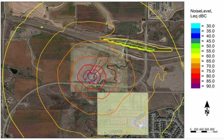
Figure 4-12 Unmitigated Fracing Location 2 Noise Contour Map (dBC)
