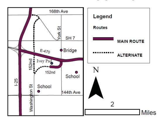
Figure 2. Map showing proposed site and truck routing. The trucks will be routed on E-470. Flowback water will be taken to disposal wells in Weld County via I-25 or US-85. Materials to be landfilled will be taken to Republic Landfill per the Waste Management Plan on file with COGCC. A Traffic Control Plan (TCP) is also being filed with Adams County, which will show signage at the site.
