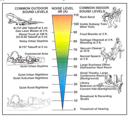
Figure 2-1 Typical Indoor and Outdoor A-Weighted Sound Levels
