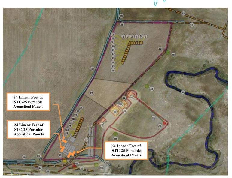
Figure 4-14 Modeled Mitigated Drilling Scenario Layout Location 2
