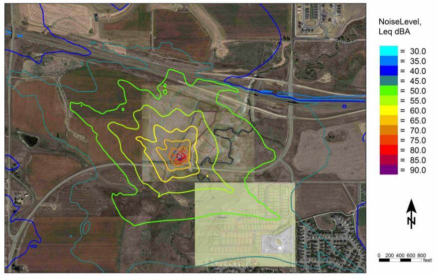
Figure 4-19 Mitigated Drilling Location 2 Noise Contour Map (dBA)
