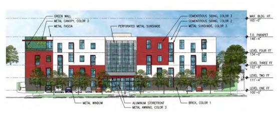
PDP elevation facing Broadway (east elevation)
