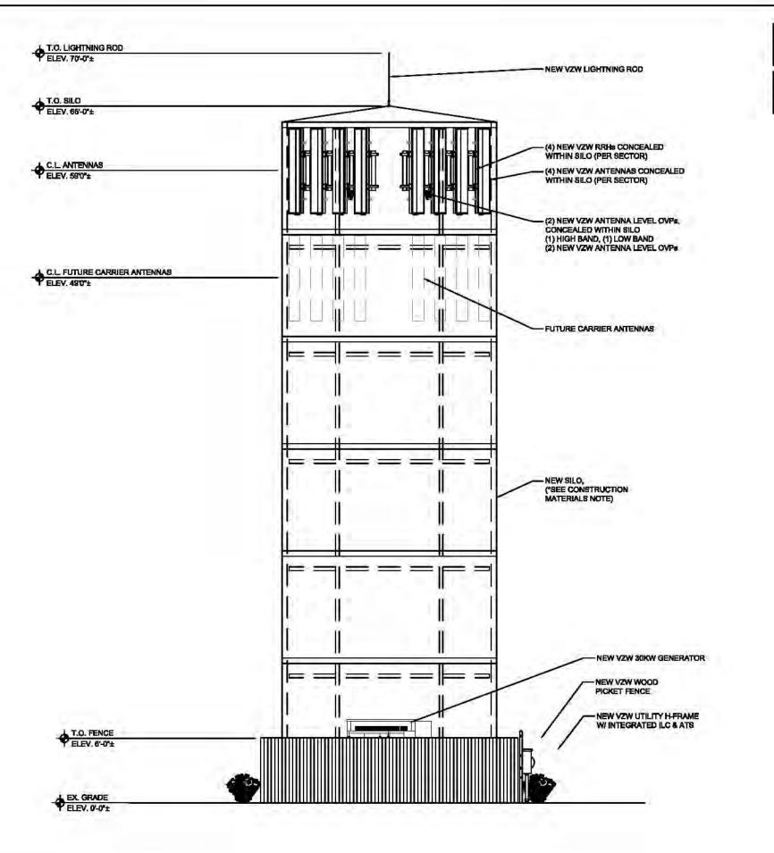
CONCEALMENT SILO STRUCTURE BY OTHERS, FINAL FRAMING AND CONFIGURATION TO BE DETERMINED
